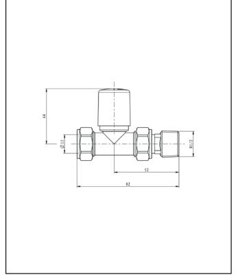
Dimensions (measurements in mm)
